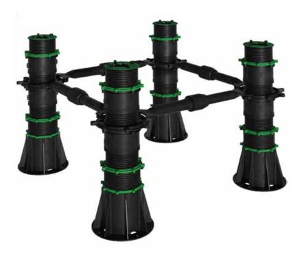
When the support reaches 800mm or more, the connecting rod makes the support more fixed. The K type is directly stuck on the K-fix collar. The SL type self-leveling needs to be matched with a big fix collar.
